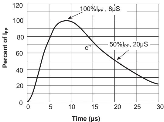
**Fig.4 Pulse Waveform-ESD(IEC61000-4-2)**
